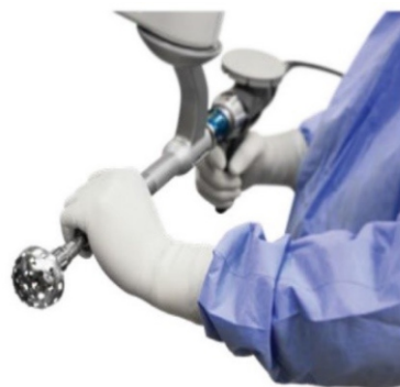
Figure 1: MAKO robotic arm is affixed to an acetabular reamer to deliver input and direct the surgical reaming of the acetabulum throughout the procedure. 17
